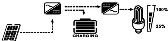
Solar power can supply power to the load while charging the battery.
